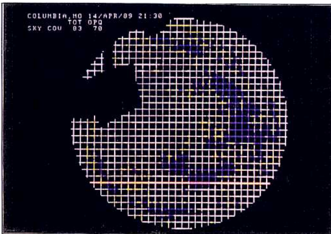
Fig. 4. Sample One-Minute Cloud/No cloud Decision Image. This shows the subset saved at 1 minute intervals.
